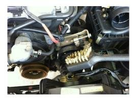
Use the brass brush to scrub off the pulleys, especially if there is lots of gunk. Some people have used brake pad cleaner if they are really nasty. Brass is important because a steel brush can possibly score the pulleys, which wear the belts faster.
