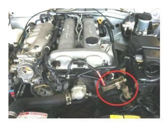
The belt closest to the radiator goes from the engine to the air conditioner compressor then the power steering. Not all miatas have this belt depending on A/C on power steering. The tension in this belt comes from the air conditioner compressor pulley. The tensioner (circled) needs to be adjusted to remove the belt.
