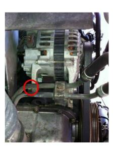
Use a 14mm wrench to loosen bolt 2. Get up and dust yourself off. Loosen bolt 3 with a 12mm socket to move the alternator. If you just want to tighten this belt, then skip down to the next page. Slip off the belt.
