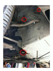
You can get away with just removing the fasteners on the passenger side of the splash guard to access bolt 2. There should be 10mm bolts and Philips head screws holding it up. The left photo shows about where the bolts are (taken from below the car in front of the passenger tire, looking up). On the right shows the location of bolt 2 after the splash guard is moved (behind the coolant line).
