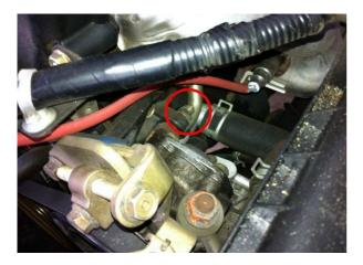
You may need to secure the nut on opposite end of bolt 2. Use a 14mm wrench on the nut circled (photo looking over the top of the tensioner into engine compartment).
