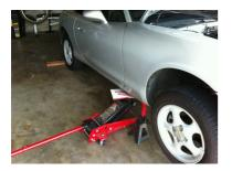
Setup your car. Jack the front wheels and put them on stands. Cardboard on the jack can help prevent dents in the metal. Make sure the parking break is on and that you block the rear wheels. Leaving the jack extended on one gives you added insurance.
