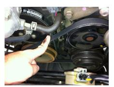
Tighten bolt 3 while checking the tension on the belt with your finger. The belt should be tightened so that 22 lbs causes 1/3 inch deflection. Tighten bolt 2 then bolt 1.
