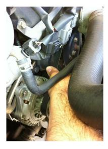
Put the new belt on the alternator loop. First wrap it around the water pump pulley, then the engine pulley (the grove closest to the engine) and lastly around the alternator. As you tighten bolt 3, check the tension on the belt with your *calibrated* finger. The belt need to be tightened so that 22 lbs causes 1/3 inch deflection. If you don't trust your finger, then you can get a belt tension gauge like the one to the right.
